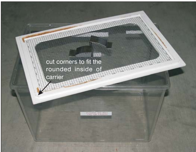
... and the bottom of the lid showing the cut corners on the stiffeners to fit the rounded edge of the carrier. Photo ©2013 Karen Robbins.
