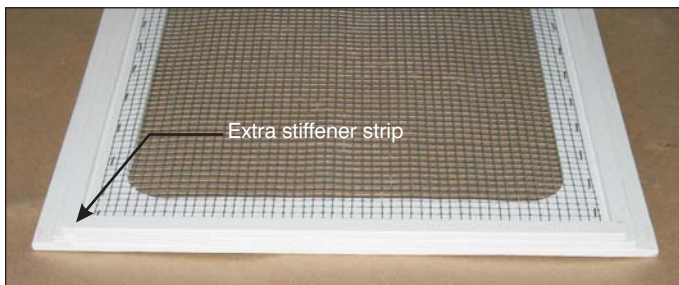
This section of lid used on a 60-gallon tank that butts up to another section of lid showing the extra stiffener strip added on top of the other strips for extra strength. Photo ©2013 Karen Robbins
