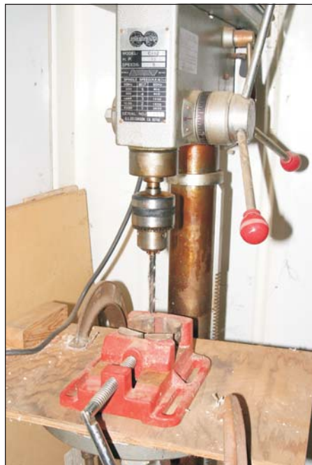
Drill press with \frac{3}{8} " bit and small vise to hold pieces of wood in place while the hole is being drilled.
